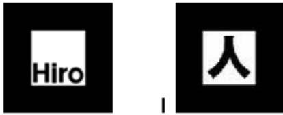
Fig 9: Hiro and Kanji, our two place markers for the NyARToolkit to track tokens.
