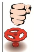
Fig 5: Bumping Motion to Insert Valve
